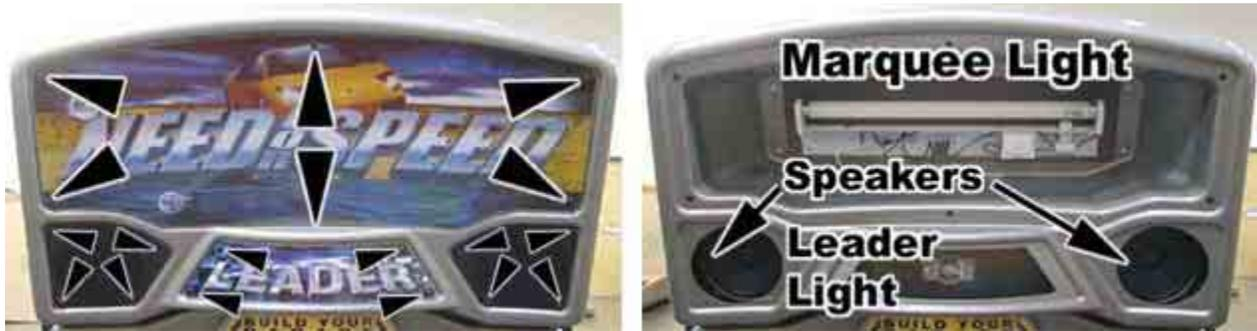
To gain access to the light bulbs and speakers behind the marquee artwork you will need a T-20H Security Torx bit for the screws. Remove the screws holding the artwork or speaker grills in place to gain access to the light bulbs or speakers in the marquee. The speaker wires can be removed from the speakers from the back side of the marquee sign.
