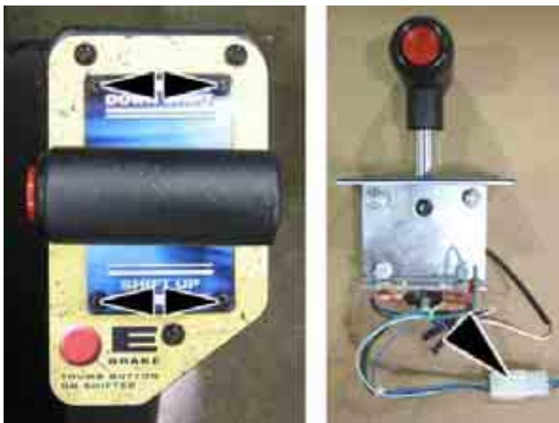
The gear shifter is one of the few items that should never break, but incase it does. To replace the shifter, remove the 4x T-10H Security Torx screws, pull up on the shifter vertically and unplug the shifter at the Molex connector.
