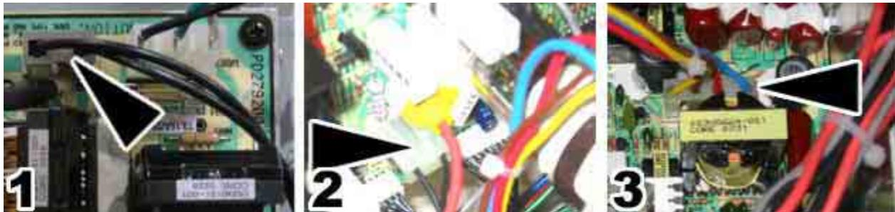
Finally you will need to unplug 2 cables from the monitor chassis PCB and 1 from the chassis neck PCB that are directly connected to the CRT shown by the arrows in the picture above.
