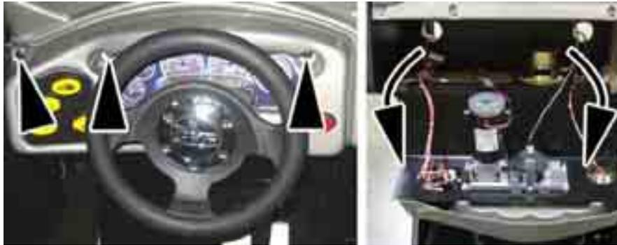
To gain access to the Force Feedback Motor and buttons remove the 3x T-25H Security Torx bolts from the top of the Driving Control Panel bezel as shown by the arrows in the picture above. The Driving Control Panel assembly is mounted to a hinge and will fold down.
