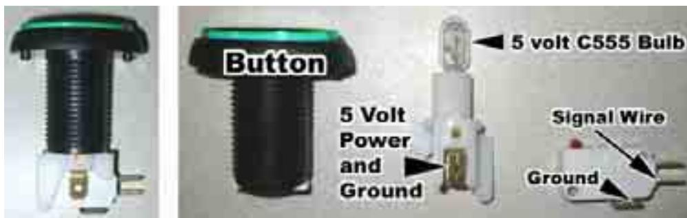
The buttons on the NFS cabinets are illuminated with 5 volt C555 bulbs. To replace the bulbs and micro switches open the Driving Control Panel assembly. Gently rock the white plastic bulb house from side to side to loosen it from the button housing. When reconnecting the wiring to the micro switch and bulb do not connect the 5 volt power wire to the micro switch as this will damage the computer and other electrical hardware connected to the wiring harness.
