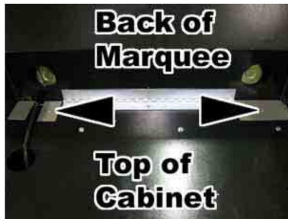
Next remove the 3x T-25H Security Torx screws holding the Driving Control Panel assembly and lower the assembly down. At the top of the cabinet fold the Marquee forward and remove the two Phillips screws holding the top of the monitor cover to the cabinet.
